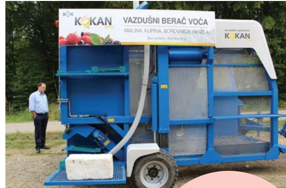
Figure 11: Mechanized raspberry harvesting with trailed harvester.
