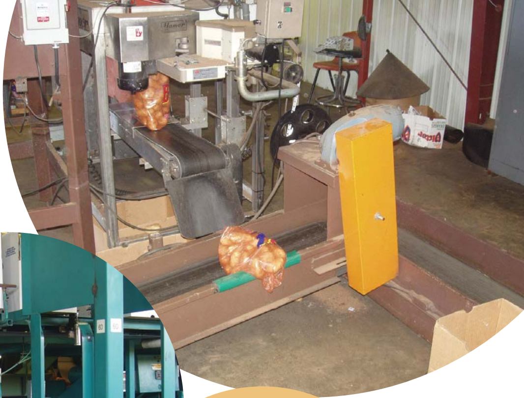
Figure. 9: The sorted tubers are automatically packed either in plastic bags (on the left) or cardboard boxes (on the right). The packaging is connected to a scale, and tubers are funnelled into it until it reaches the desired weight. Once the required weight is reached, the full packaging is replaced, and the empty one takes its place. The entire process is fully automated, minimizing the human role in supervising the machine operations.
