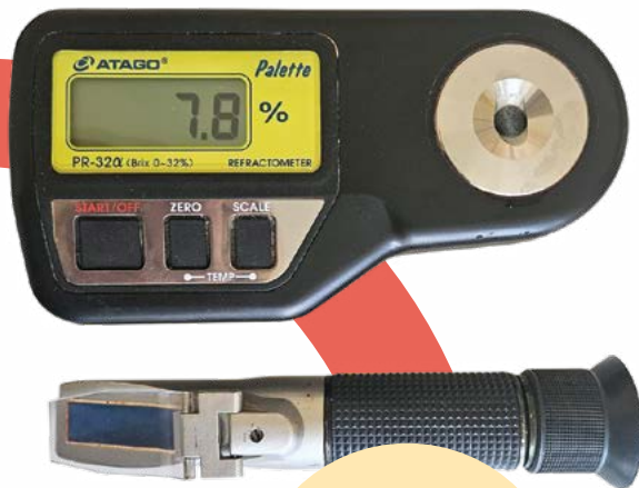
Figure 3 Digital and analogue (manual) refractometer
